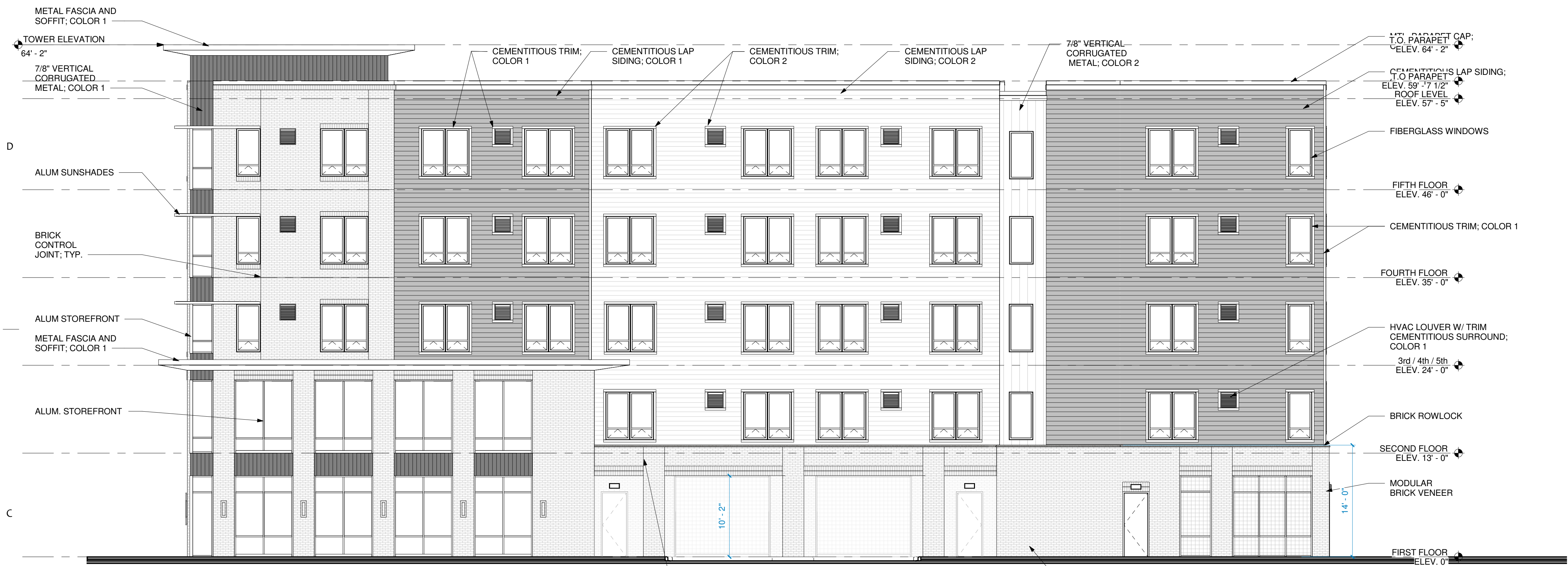
1 SOUTH ELEVATION SCALE: 1/8" = 1'-0" FENESTRATION PERCENTAGE CALCS: (942.795SF/1,859.340SF) = 0.51%
