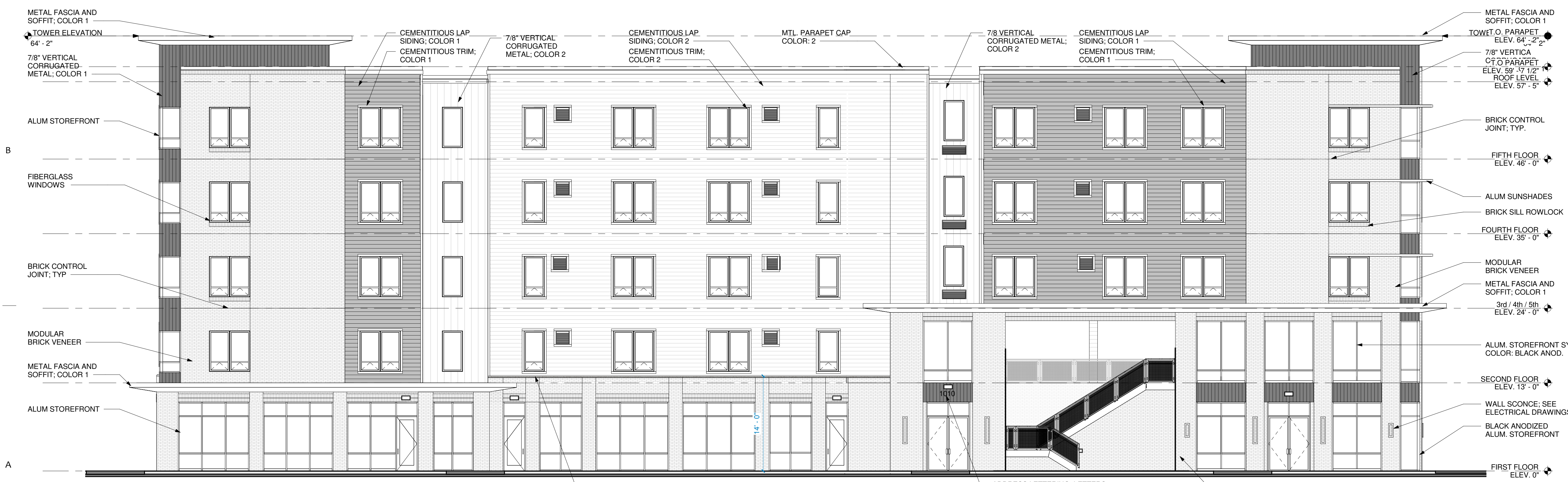
2 WEST ELEVATION SCALE: 1/8" = 1'-0" FENESTRATION PERCENTAGE CALCS: (1,424.755SF/2,422.29SF) = 0.59%
